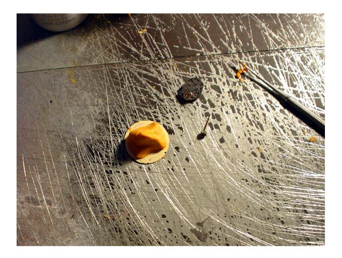
Next, turn the dial over and place the dial and putty on the Speedi-fit container lid. Press down on the dial so that the putty is around 3.7mm thick, or as thick as the stock movement holder should be.
