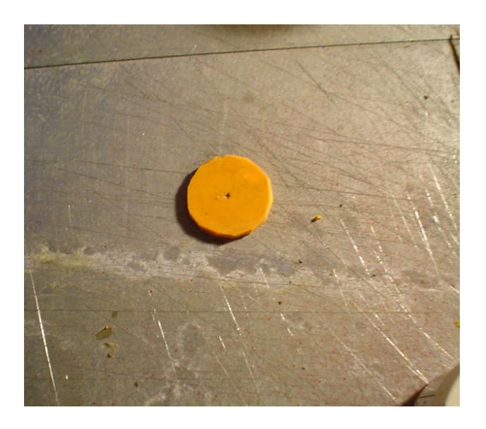
Use your Dremel tool to smooth out the movement holder and remove putty around the edges, so that the watch case back is able to engage the case threads. You can find the Dremel Multipro kit at hardware stores for around \$45, or you could look for a used one on Ebay. This tool comes in handy for all kinds of projects. It's definitely worth looking into.
