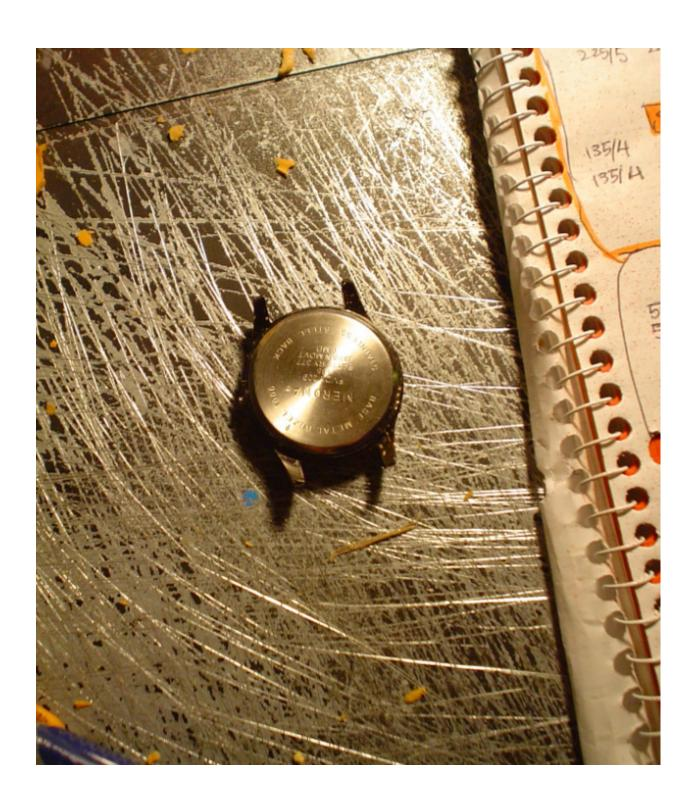
Here is an example using only measurements. Mix up some Speedi-fit and flatten it out. All you need to know is the diameter of the movement, and the diameter of the inside of the watch case.
