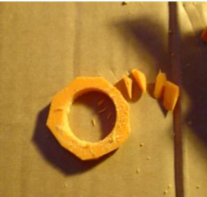
Cut out the shape of the movement holder with a razor blade or utility knife. Use your Dremel tool to perfect the shape.
